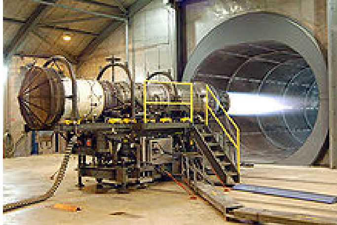
Figure 7: A Pratt & Whitney F100 jet engine is being tested (WK1, 2015).
