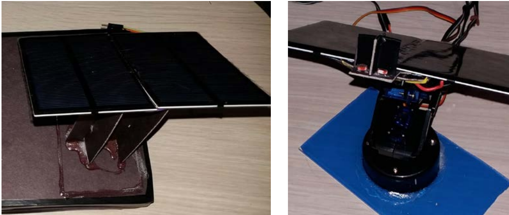
Figure 1. Fixed system(a), tracker system(b)
