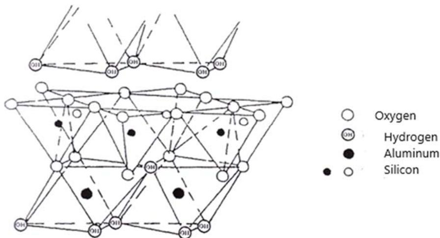
**Figure 2.** Structure of kaolinite
