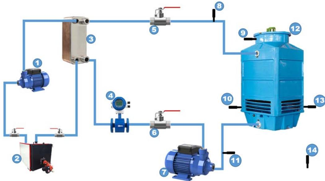
**Figure 1.** Experimental setup. 1: Boiler line water pump, 2: Gas fired hot water boiler, 3: Plate heat exchanger, 4: Flowmeter, 5-6: Flow control valve, 7: Cooling tower water pump, 8-9-11-14: Thermocouples, 12: Cooling tower, 10-13: Wet bulb temperature measuring devices.
