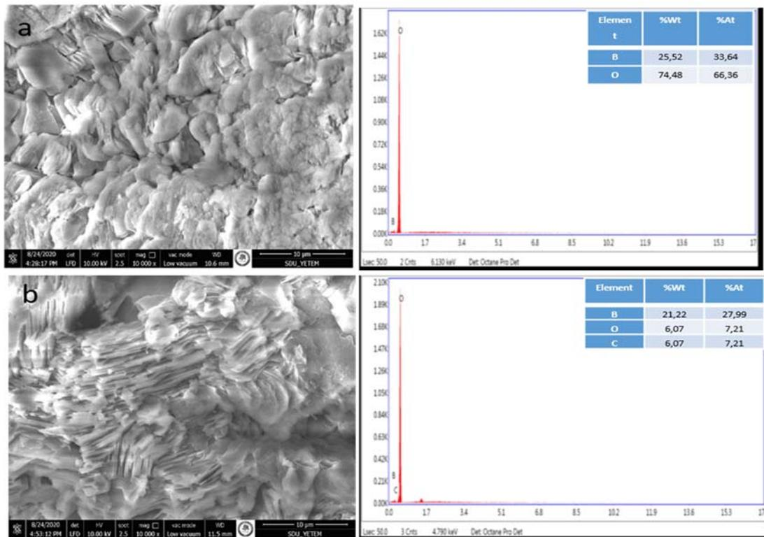
**Figure 3.** SEM/EDS Results of a) H<sub>3</sub>BO<sub>3</sub> and b) H<sub>3</sub>BO<sub>3</sub> doped GO
